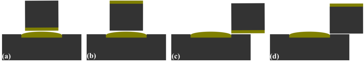
Figure 6 Types of part-site contacts. (a) Contact between binding surfaces, also labeled as an “assembly contact”. (b) Contact between a site and the non-binding surface of a part. This is labeled as incorrect assembly contact. (c) and (d) are contacts when a part lands outside of a site.
